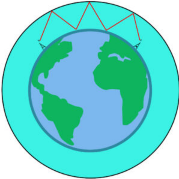
Signals being refracted by ionosphere.
